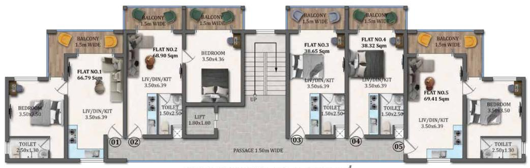
TYPICAL FLOOR PLAN( 1st TO 4th FLOOR )
